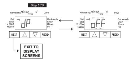
**Step 7CS** – Selecting the use of an outside signal to initiate a regeneration: Selection only matters if a connection is made to the two pin connector labeled DP SWITCH located on the printed circuit board. Following is an explanation of the options:
