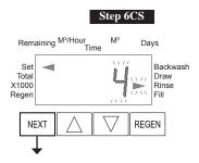
**Step 6CS** – Set duration of the special rinse cycle to be performed prior to a valve returning to Service. Selectable from 1-20 minutes or OFF. Only viewed if 50 is set in 2CS, and ALTA or ALTb is set in 5CS.
