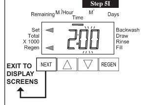
**Step 1I -** To enter Installer Display press the NEXT and **▲** buttons simultaneously for 5 seconds and release.
