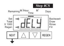
Step 4CS – Press the ▲ or  $\nabla$  buttons to select to regenerate immediately on 0 or at delayed time. Immediately on 0 can only be selected if Volume ( $M^3$ ) was selected in step 3CS and a meter must be installed. Delay is the only option for the other Step 3CS selections. Press NEXT to go to Step 5CS. Press REGEN to return to previous step.
